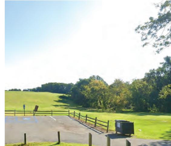
A rain garden can be installed east of the parking lot to capture and infiltrate stormwater runoff from the paved surface. A preliminary soil assessment suggests that the soils have suitable drainage characteristics for green infrastructure.
