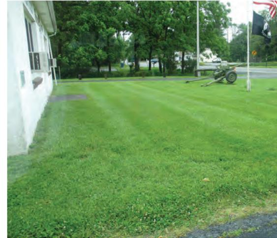
A rain garden can be installed to capture stormwater from the building's rooftop. Pervious pavement can be installed along the northwestern edge of the parking lot to capture the stormwater runoff from the parking lot. A preliminary soil assessment suggests that more soil testing would be required before determining the soil's suitability for green infrastructure.
