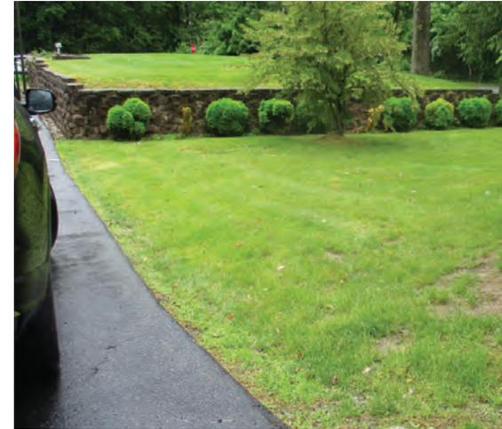
A rain garden can be installed south of the roadway to capture, treat, and infiltrate stormwater runoff from the pavement. Downspout planter boxes can be installed along the front, southern wall of the building to capture stormwater runoff from the rooftop. A preliminary soil assessment suggests that the soils have suitable drainage characteristics for green infrastructure.
